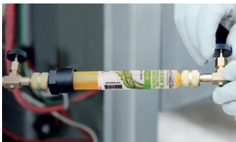
Charge inline with refrigerant
